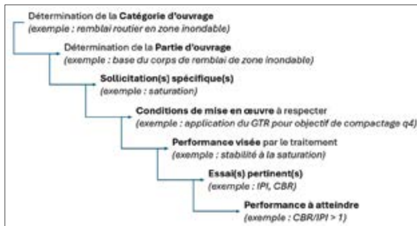
—Figure 11— Principe de la matrice Usages/ Performances.
